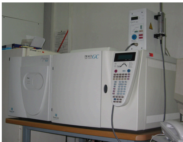
Figure -. Gas chromatography-mass spectrometry (GC-MS) is a method that combines the features of gas-liquid chromatography and mass spectrometry to identify different substances within a test sample.
